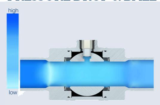
District heating systems require a minimisation of pressure losses in order to prevent additional pump performance in piping systems. Full bore valves with a straight inner geometry shows the lowest pressure losses.
